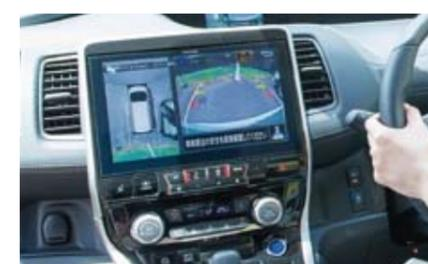
Have you had the experience where you park your car within the correct space but had no room to open the door? The system is reliable in that it shows the guiding lines to indicate the distances necessary to open and close the rear doors.
