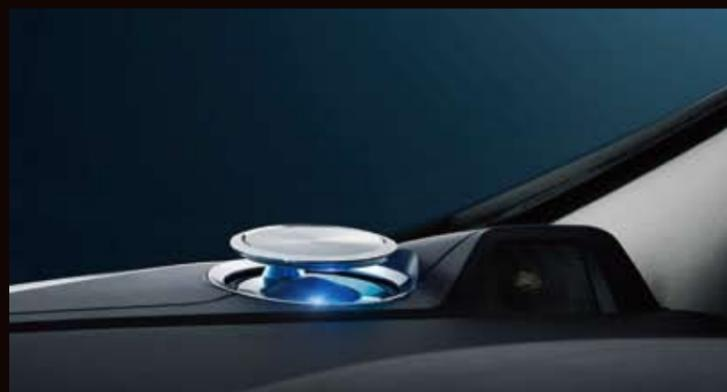
When the ignition is turned on, the active top covers and the tweeters are automatically lifted up. The high sound range from the tweeters reflects to the active top covers, causing the sound to diffuse from the dashboard.
