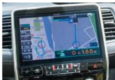
The screen shows the distance to the place to turn. Screen display simultaneously with voice makes it easy to understand.
